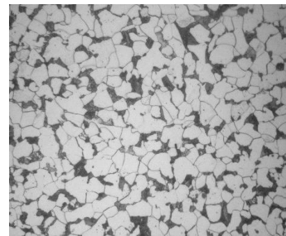
Fig. 11 Microstructure of steel (S25C)
