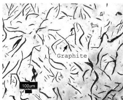
Fig. 6 Microstructure of modern machinable cast iron
