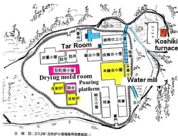
Fig. 31 Site of reverberatroy furnace in old drawing 1)
